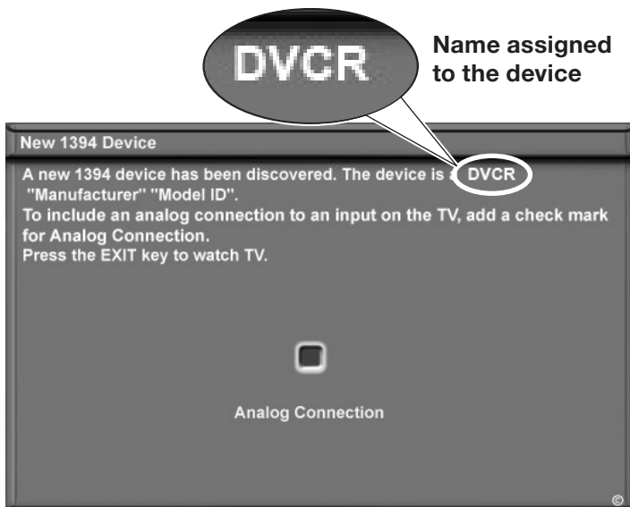
Figure 3. The ClearThought Auto Input Sensing screen for IEEE 1394 devices includes a check box for an associated analog connection.
